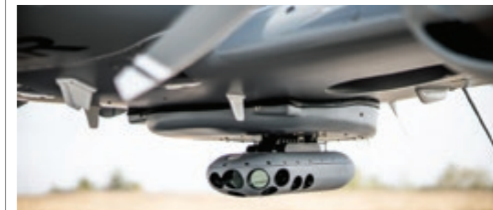
Eye in the sky: The ViDAR self-contained aerial reconnaissance (SCAR) day/night 'optical radar' pod
