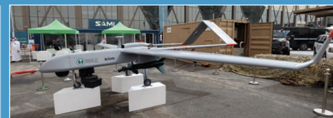
▲ The PSDRC Skyguard is on show with two 25kg munitions and an AEC EO/IR FLIR turret
