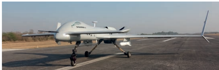
The GIDS Shahpar-II armed with two indigenous Burraq laser guided munitions. There have been at least eight firings of the weapon to date
