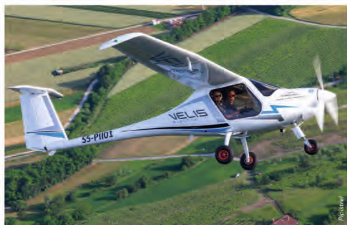
Several air forces are evaluating the all-electric Pipistrel Velis Electro two-seat trainer with a view to replacing traditionally powered types
