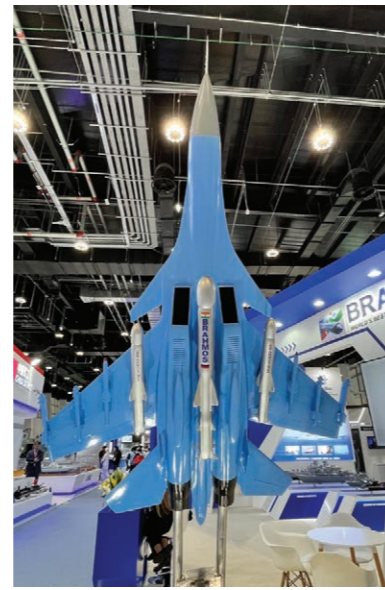
▼ The smaller NG version of Brahmos shown under the wings of a model Sukhoi Su-30, contrasting with the original version on the centreline
